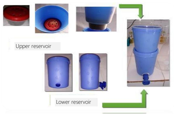
**Fig 5:** Schematization of the manufacturing steps of the two filter water jug reservoirs.
